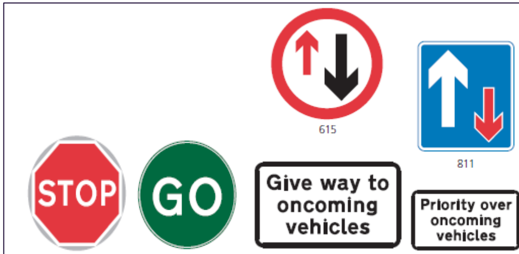
Figure 1.4: Manually operated stop/go signs and priority signs
